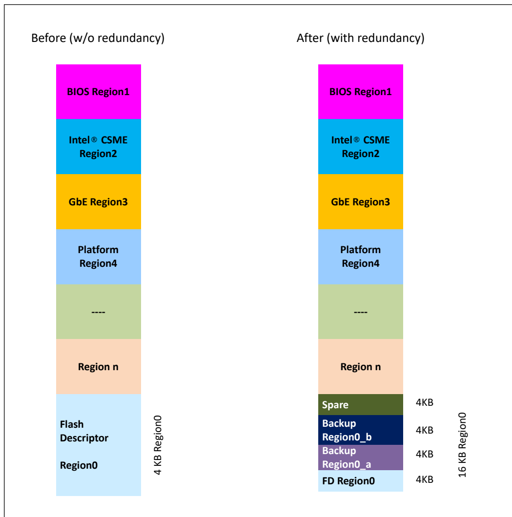
Figure 17. Flash Descriptor Redundancy
