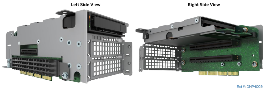
Figure 199. 1U Standard Riser Card
