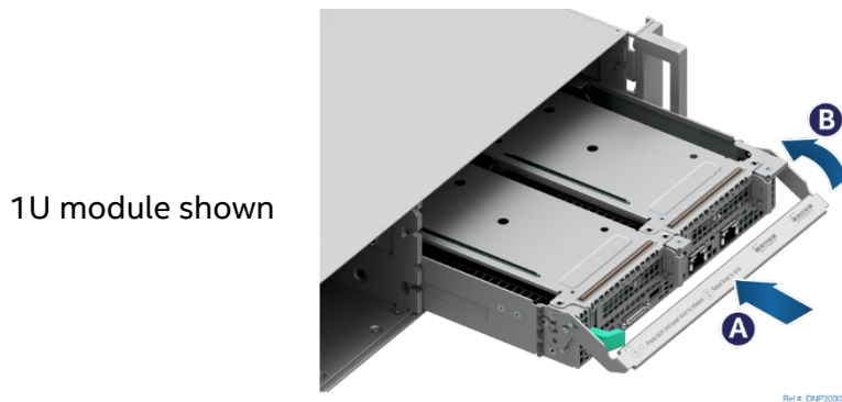
Figure 136. Installing a Module
