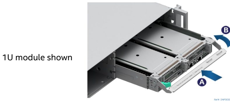
Figure 53. Installing a Module
