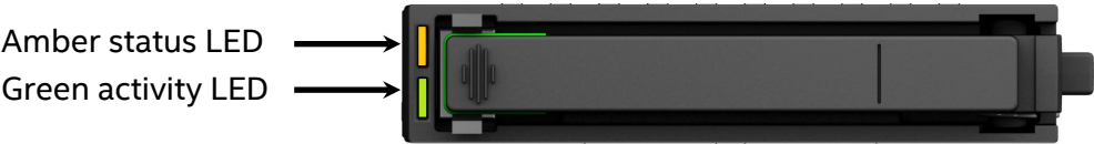
Figure 55. Drive Carrier LED Identification
