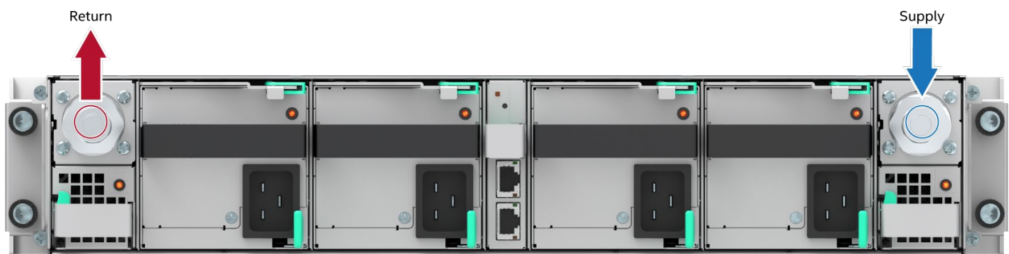
Figure 76. Chassis Plumbing Couplings Identification
