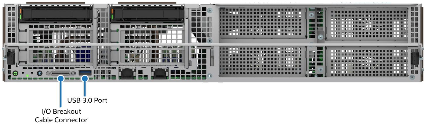
Figure 68. USB Port Location – 2U PCIe* Accelerator Module
