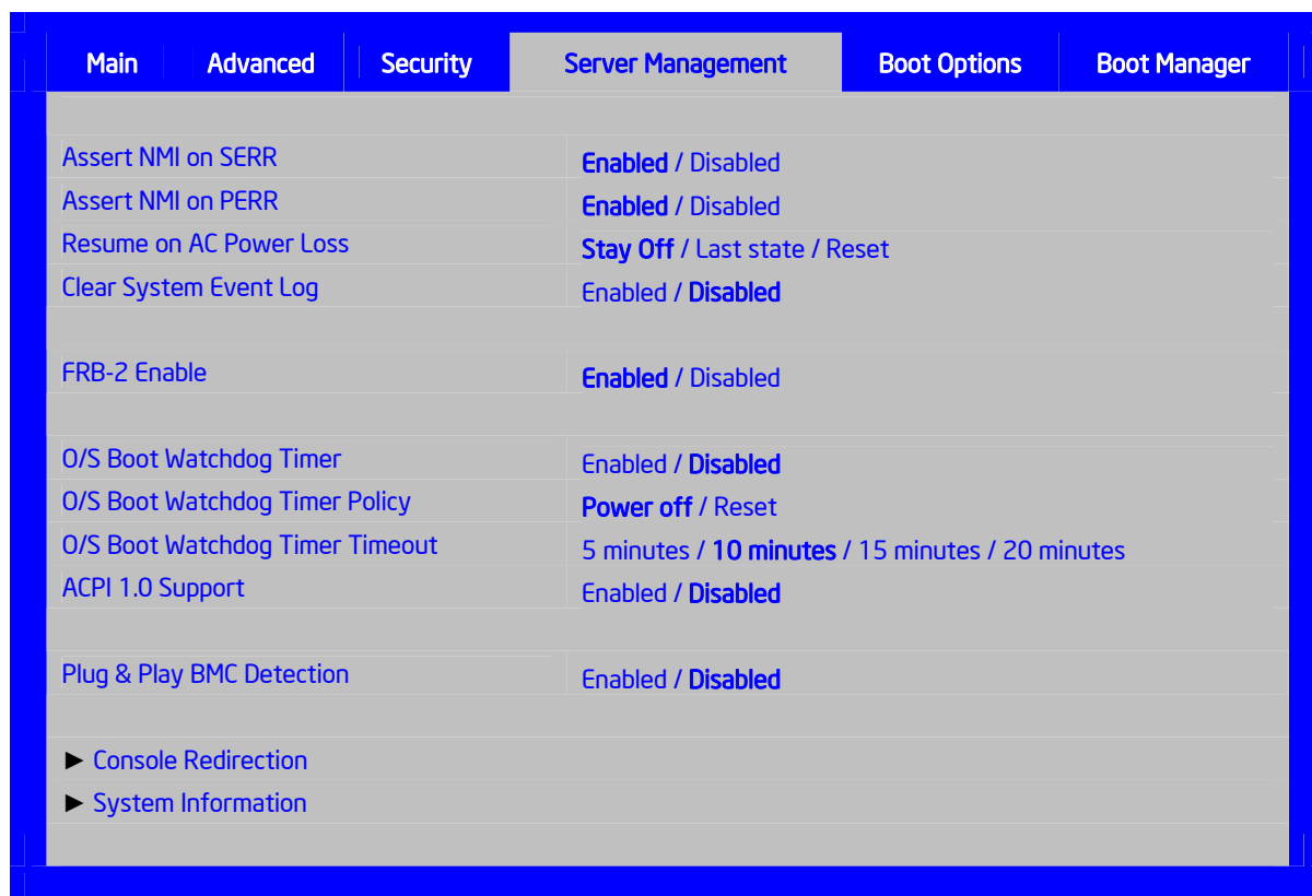
Figure 41. Setup Utility — Server Management Configuration Screen Display
