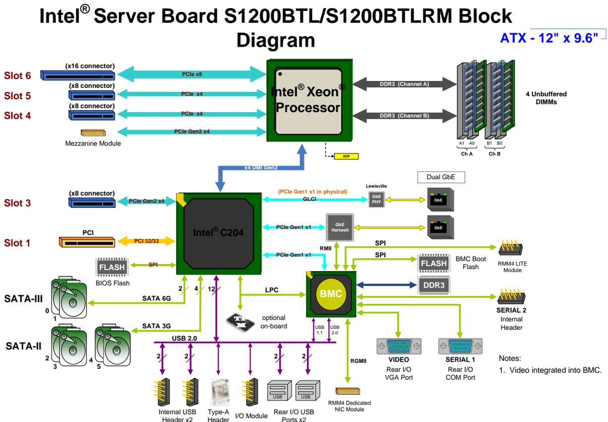
Figure 11. Intel® Server Board S1200BTL/S1200BTLRM Functional Block Diagram
