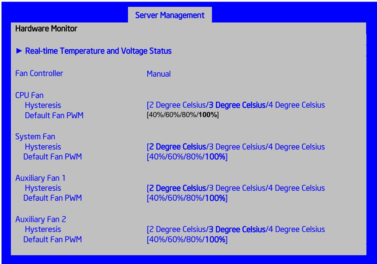
Figure 32. Hardware Monitor Screen, Manual Fan Control (S1200BTS)
