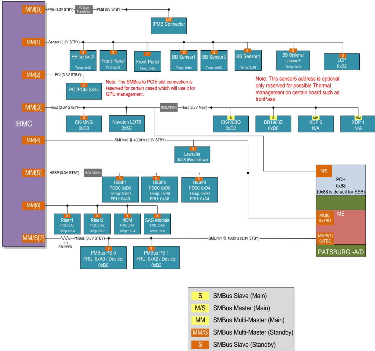
Figure 14. Server Management Bus (SMBUS\*) Block Diagram
