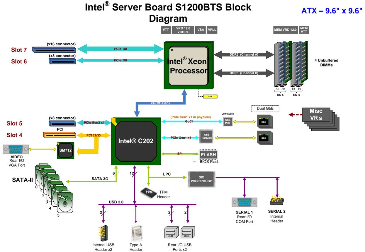
Figure 12. Intel® Server Board S1200BTS Functional Block Diagram
