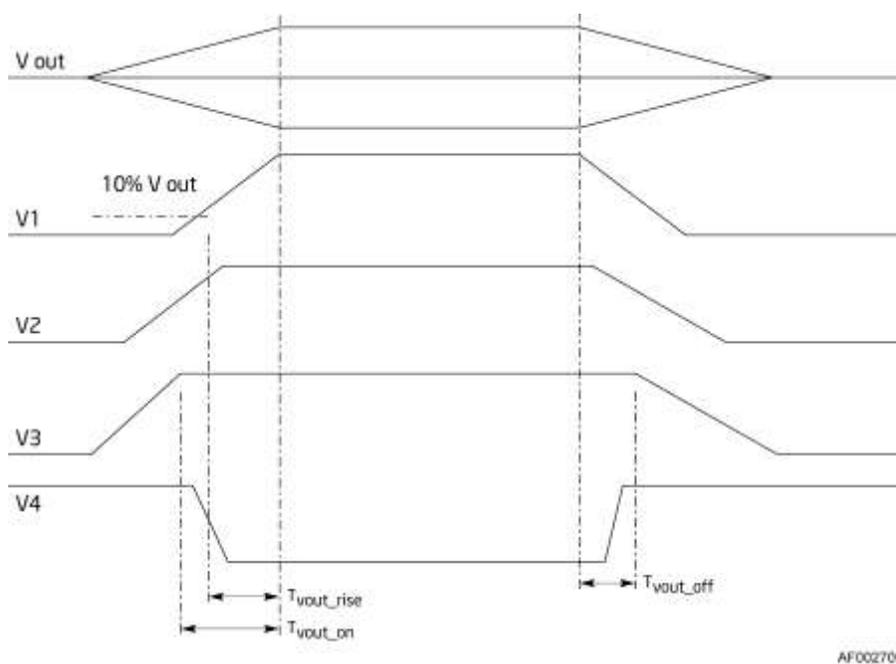
**Figure 49. Output Voltage Timing**
