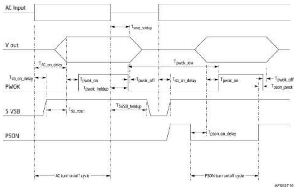
Figure 50. Turn On/Off Timing (Power Supply Signals)
