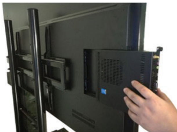
Figure 1. Open Pluggable Specification compute modules for interactive flat panel displays.
