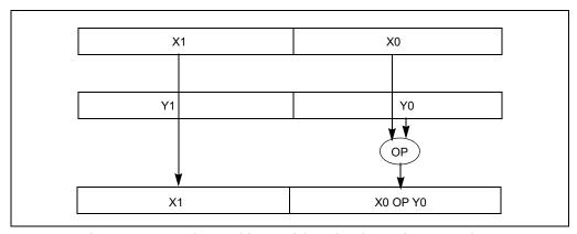
Figure 11-4. Scalar Double Precision Floating-Point Operations
