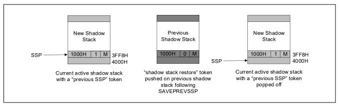
Figure 17-3. SAVEPREVSSP to Save a Restore Point
