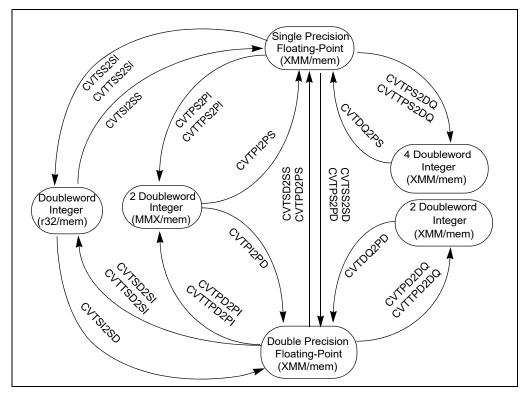
Figure 11-8. Intel® SSE and SSE2 Conversion Instructions
