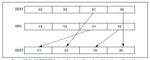
Figure 10-9. UNPCKLPS Instruction, Low Unpack and Interleave Operation
