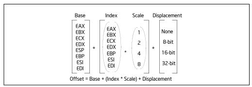
Figure 3-11. Offset (or Effective Address) Computation
