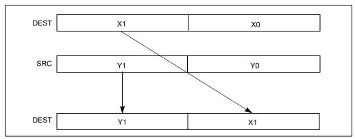
Figure 11-6. UNPCKHPD Instruction, High Unpack, and Interleave Operation
