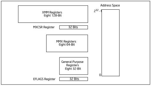
Figure 11-1. Intel® Steaming SIMD Extensions 2 Execution Environment
