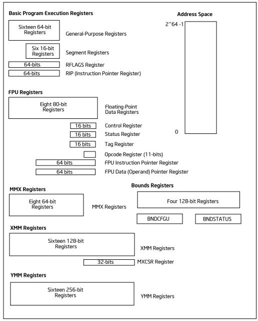
Figure 3-2. 64-Bit Mode Execution Environment
