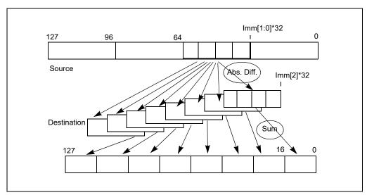
Figure 12-4. MPSADBW Operation
