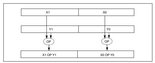
Figure 11-3. Packed Double Precision Floating-Point Operations
