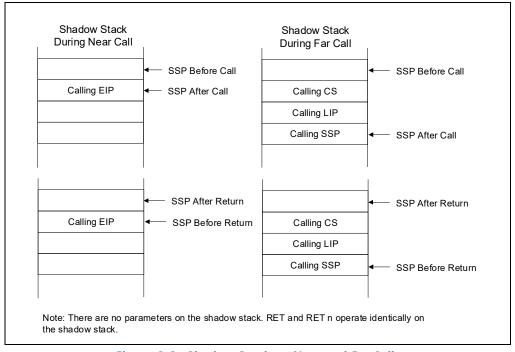
Figure 6-3. Shadow Stack on Near and Far Calls
