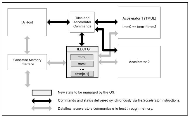
Figure 18-1. Intel® AMX Architecture
