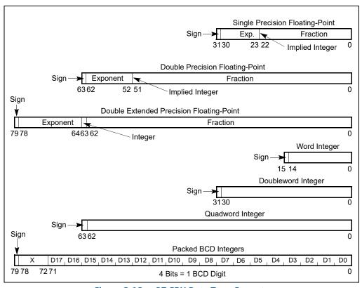
Figure 8-13. x87 FPU Data Type Formats
