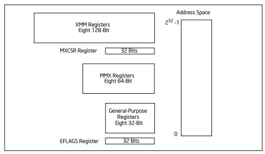
Figure 10-1. Intel® SSE Execution Environment
