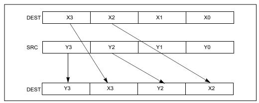
Figure 10-8. UNPCKHPS Instruction, High Unpack and Interleave Operation
