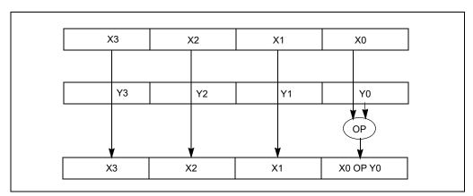
Figure 10-6. Scalar Single Precision Floating-Point Operation
