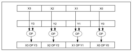
Figure 10-5. Packed Single Precision Floating-Point Operation
