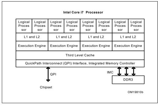
Figure 2-8. Intel® Core™ i7 Processor
