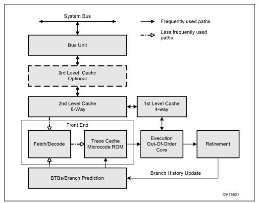
Figure 2-2. The Intel NetBurst® Microarchitecture
