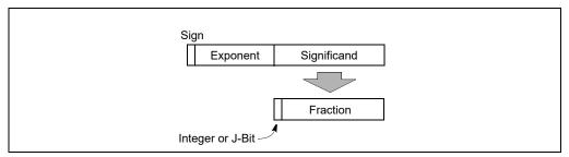
Figure 4-11. Binary Floating-Point Format
