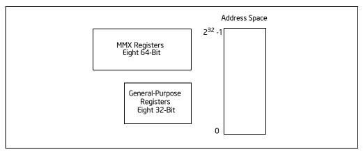
Figure 9-1. MMX Technology Execution Environment
