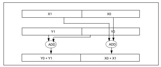
Figure 12-2. Horizontal Data Movement in HADDPD
