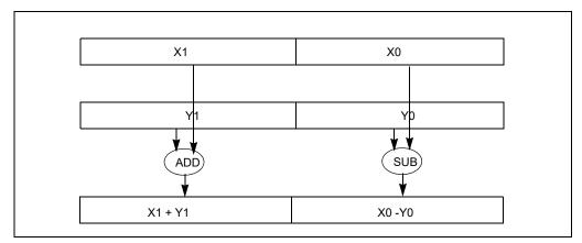
Figure 12-1. Asymmetric Processing in ADDSUBPD
