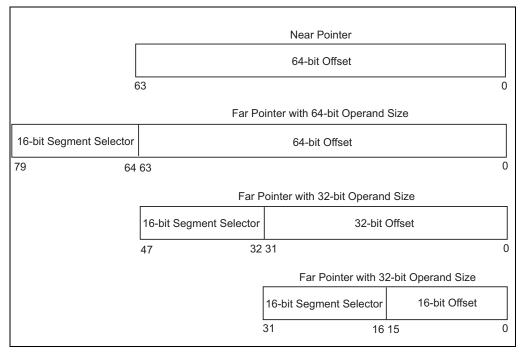
Figure 4-5. Pointers in 64-Bit Mode
