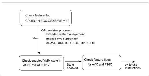
Figure 14-3. General Procedural Flow of Application Detection of Float-16
