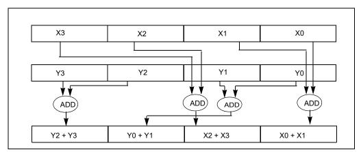
Figure 12-3. Horizontal Data Movement in PHADDD
