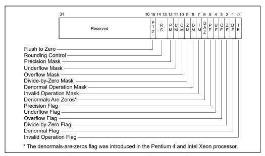
Figure 10-3. MXCSR Control/Status Register
