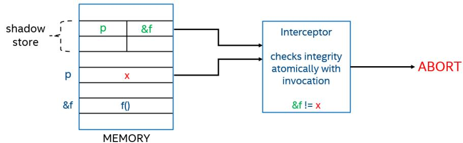
Simplified Illustration: integrity check upon function pointer invocation determines that a function pointer has been corrupted relative to its shadow copy and gracefully aborts – the discrepancy is that the pointer 'p' no longer points to 'f' as it should
