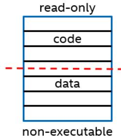
Simplified Illustration: memory is separated into code and data, the former being executable but not modifiable, the latter being modifiable but not executable
