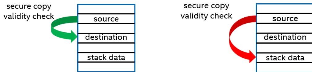
Simplified Illustration: validity check allows a source buffer to be copied to a legitimate destination (left pane), but not to a sensitive destination (right pane)
