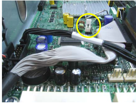
Close up of revised IDE cable fold & original BBSJ
