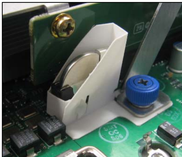
Figure 4. Battery Isolation in Place
