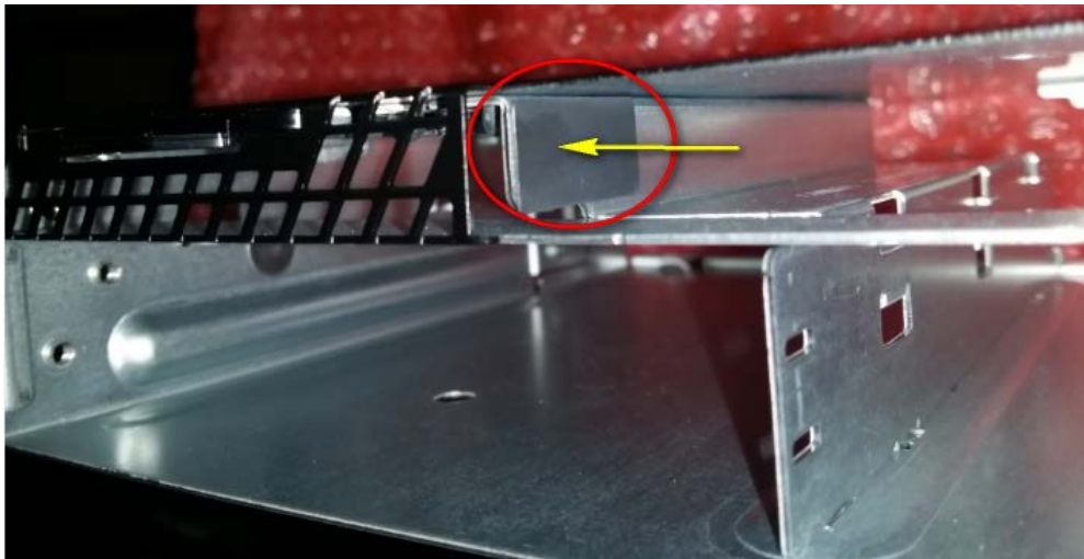
Example of the mylar bumper on the side of the optical drive bay
