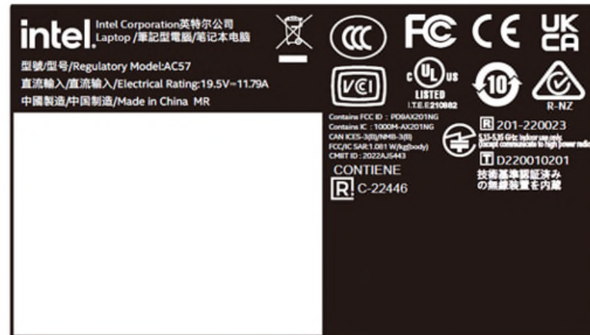
230W system rating label (before)
