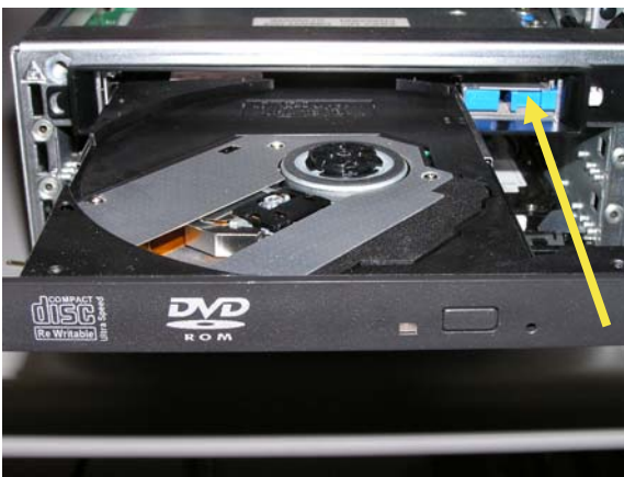
Optical drive can be removed by moving the lever to the left (see yellow arrow). The lever can be moved with a finger or general tool (like a screwdriver).
