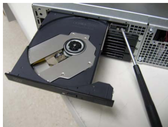
Optical drive can be removed by moving the lever to the left (see yellow arrow). The lever can be moved with a finger or general tool (like a screwdriver).
