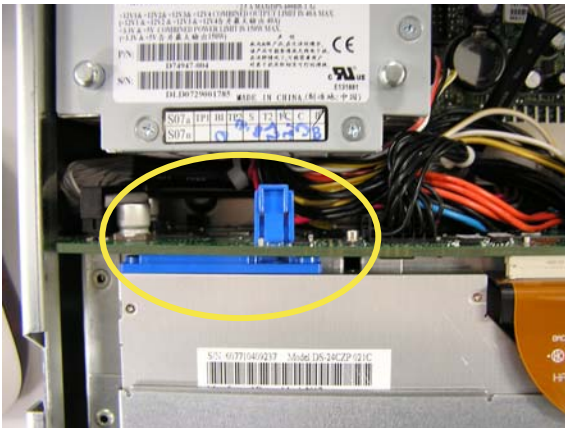
Optical drive installed via original retention mechanism shown on left.
