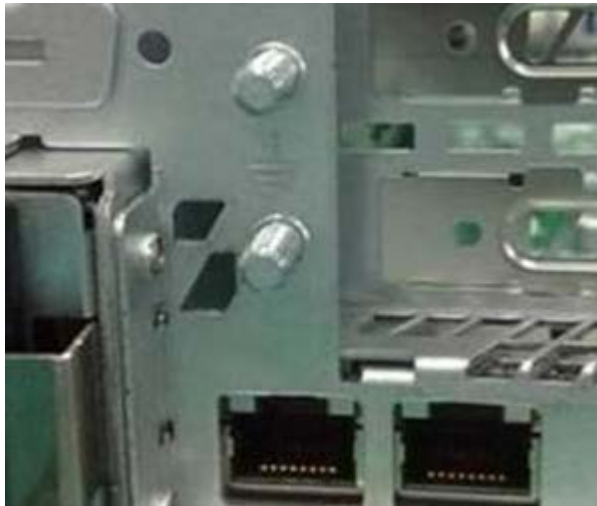
Figure 1: The ground studs
