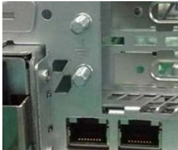
Figure 1: The ground studs
