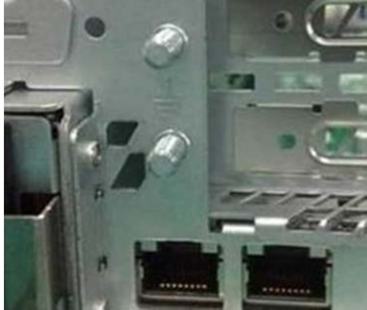
Figure 1: The ground studs
