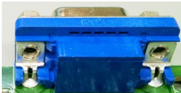
Alternate VGA connector (riveted)
