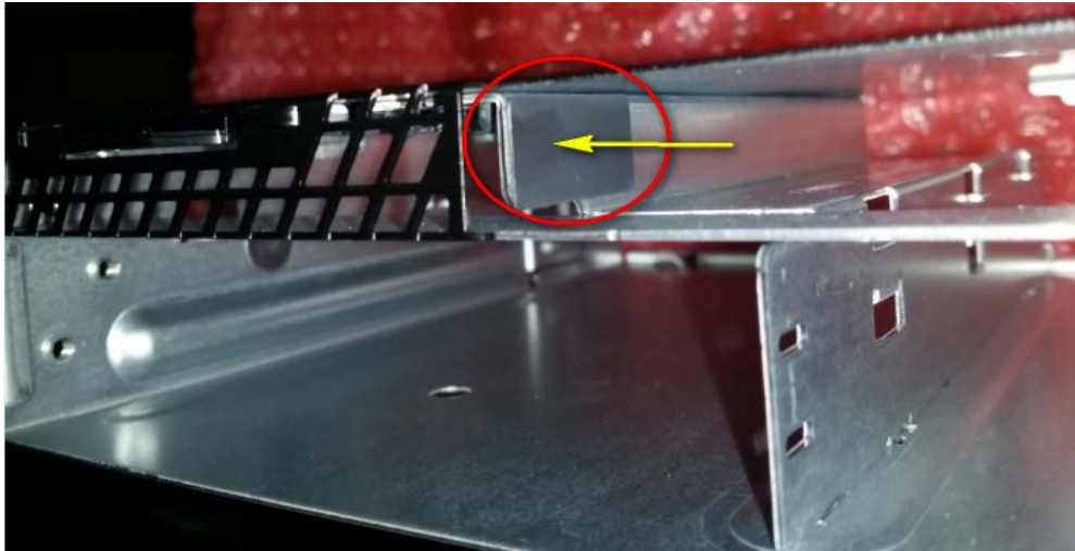
Figure 1. Example of the mylar bumper on the side of the optical drive bay
