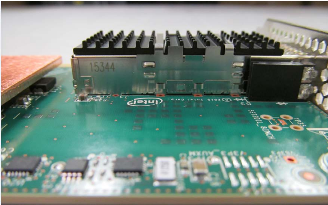
Properly Seated QSFP cage assembly
