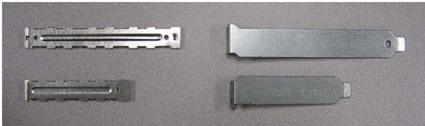
Old PCI Filler Panels
