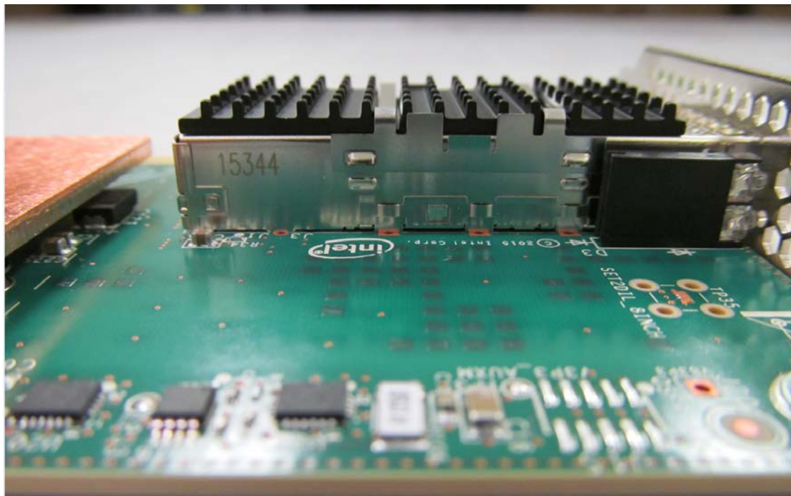
Properly Seated QSFP cage assembly
