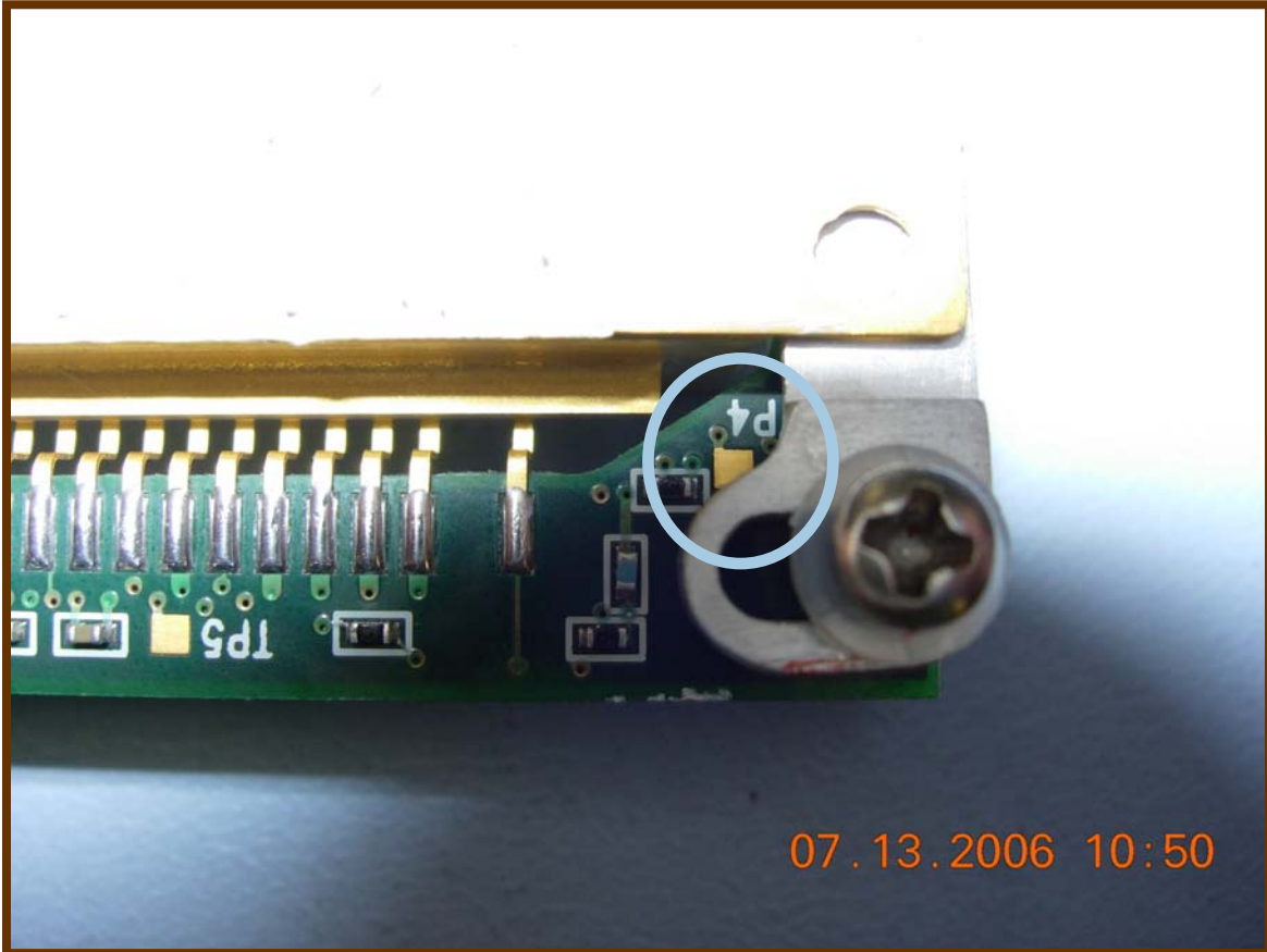
Short of TP4 to metal bracket
