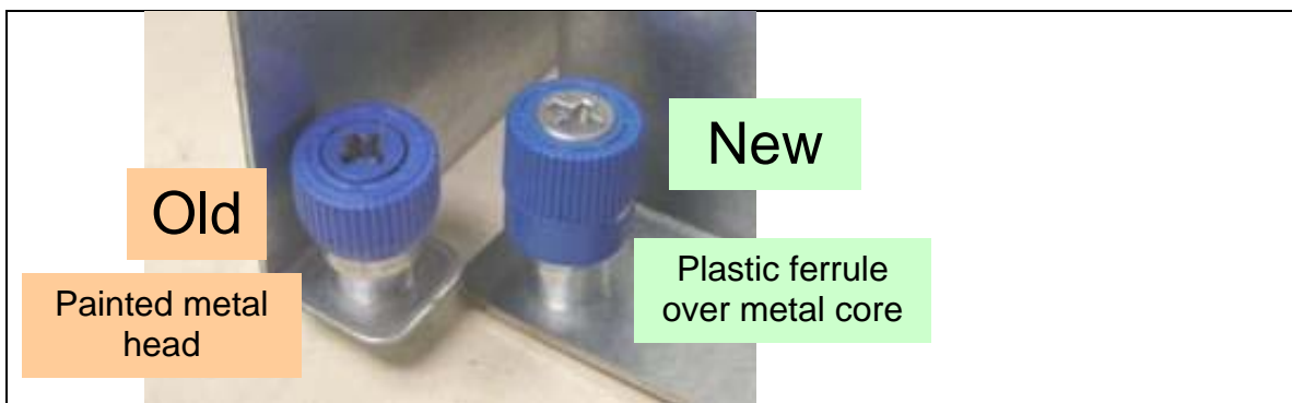
Figure 3. Change to Captive Screw on PCI riser assembly
