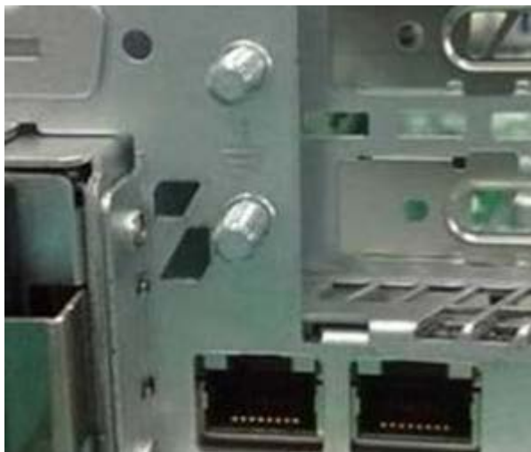
Figure 1: The ground studs
