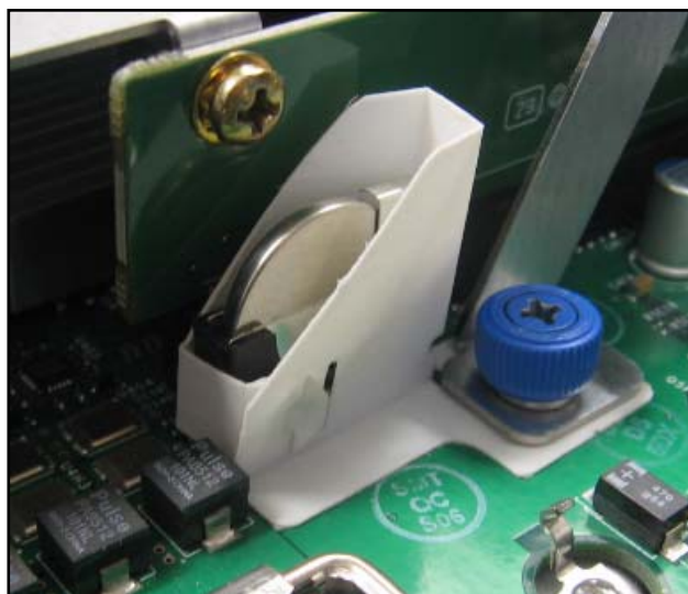
Figure 2. Battery Isolation in Place
