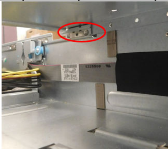
Image 1. Before Change - Chassis with EMI clips
