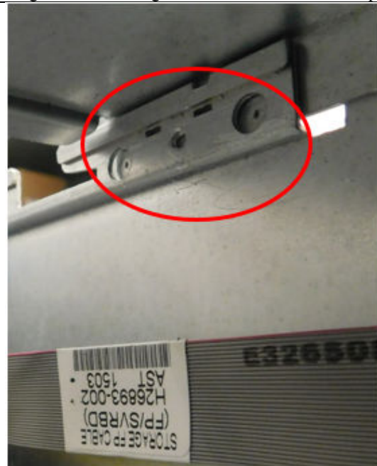
Image 2. After change - Chassis without EMI clips
