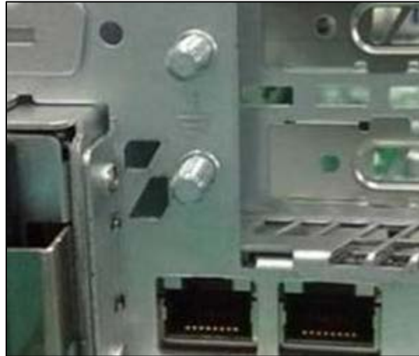
Figure 1: The ground studs
