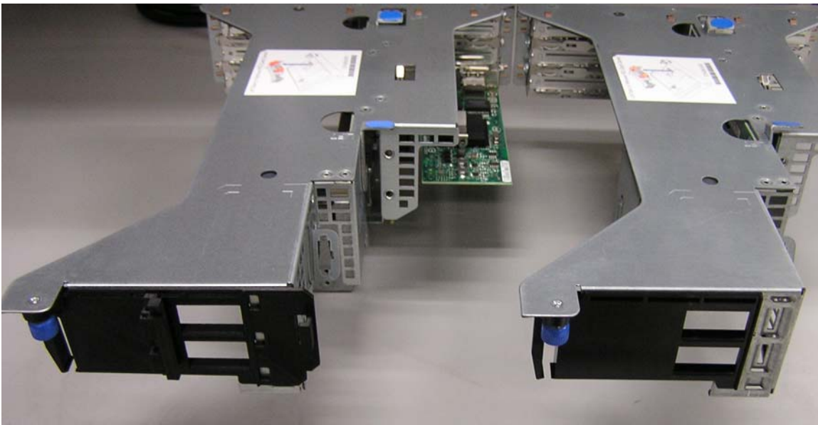
Revised PCI board retention bracket
