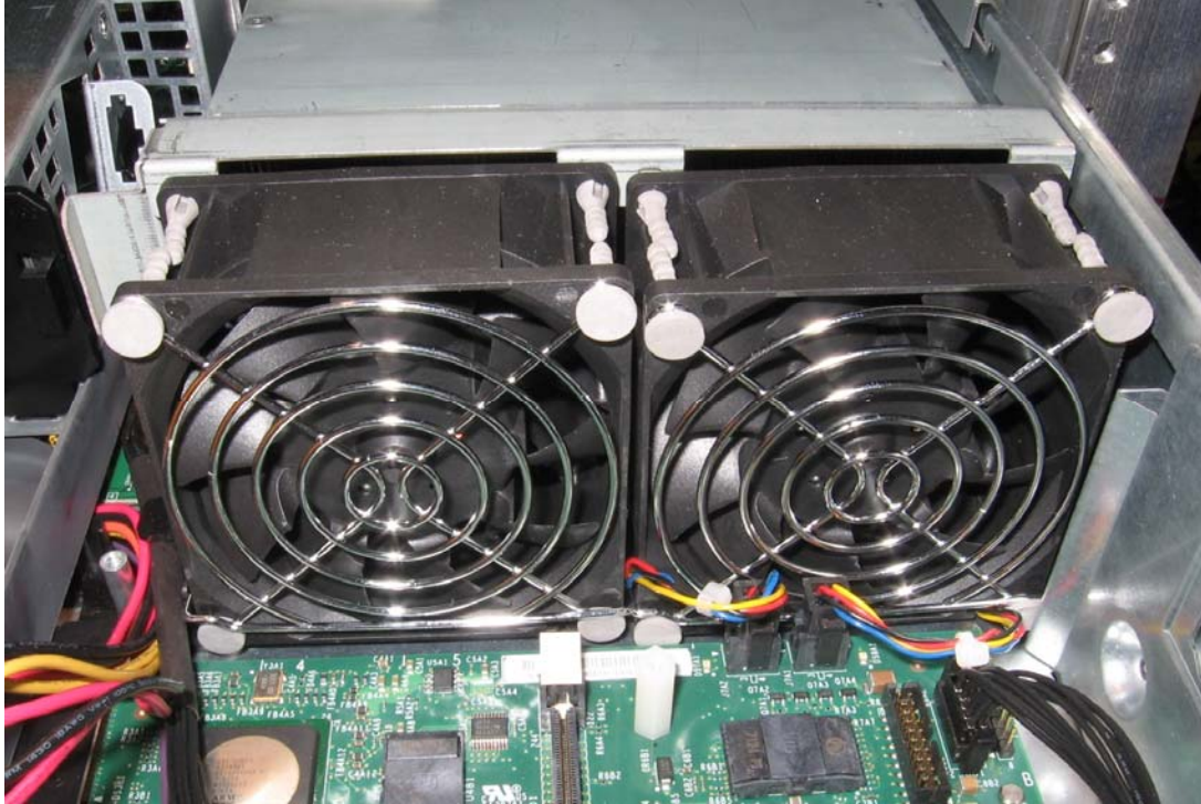
Revised 80mm fan assemblies and revised CPU air duct installed with top cover removed
