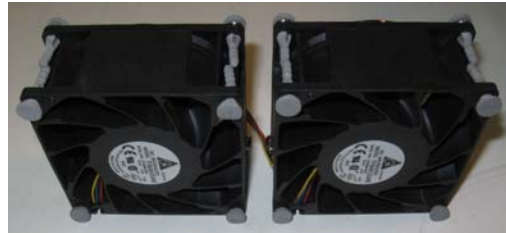
Revised 80mm fan set (CPU side)
