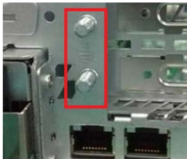
Figure 1: The ground studs
