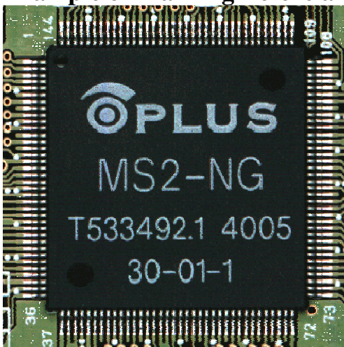
Old inked marking of molded package surface.
