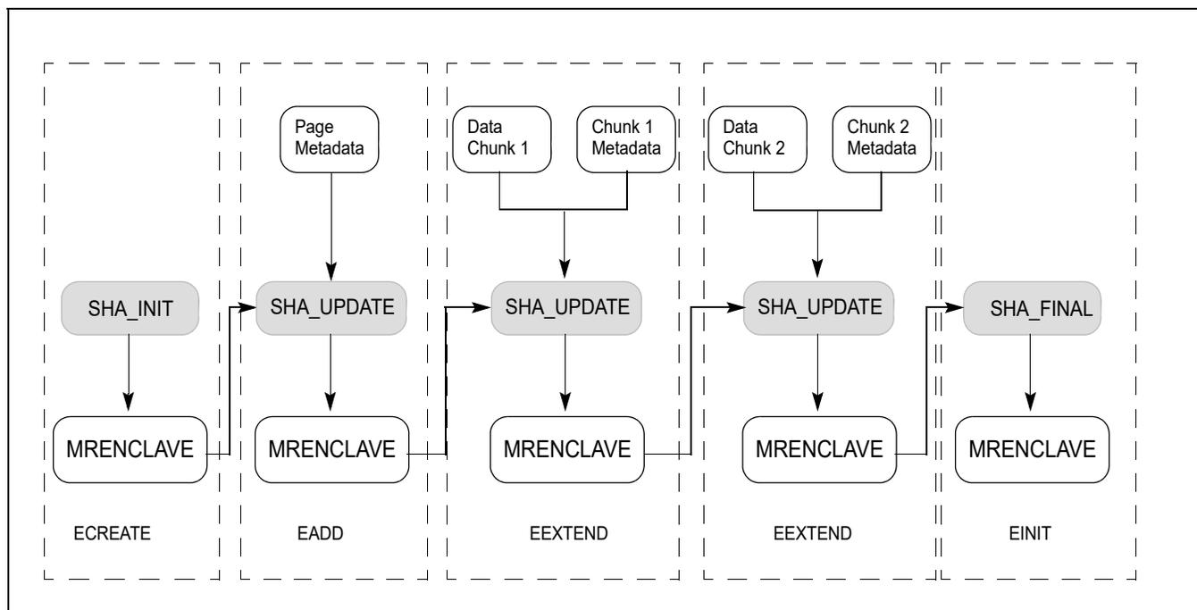
Figure 36-2. Measurement Flow of Enclave Build Process
