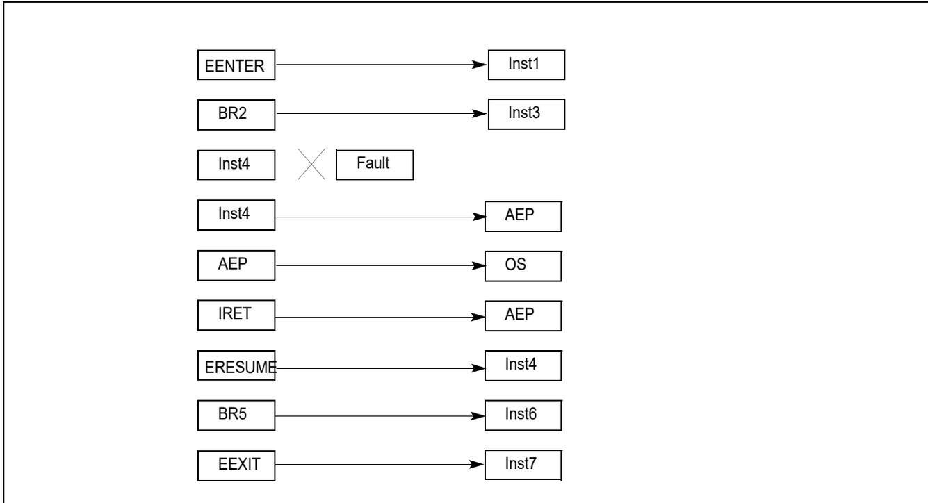
Figure 40-3. LBR Stack Interaction with Opt-in Entry
