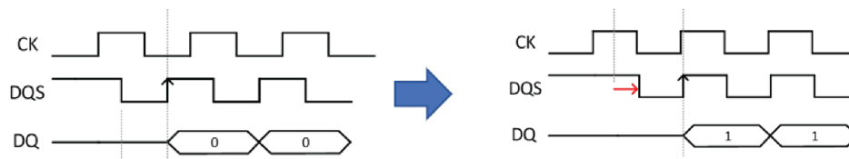
Figure 39. DQS and MEM_CLK are phase aligned when 0 to 1 transition is detected on DQ pins
