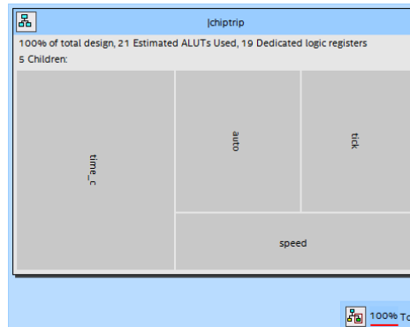
Figure 70. Top-Level Entity in the Design Partition Planner
