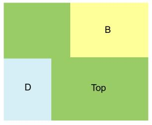
When working with the Quartus II software, designers can create configuration files for each of the source files that represent different functions in each reconfigurable design partition. The device can be reconfigured with any combination of these files.
