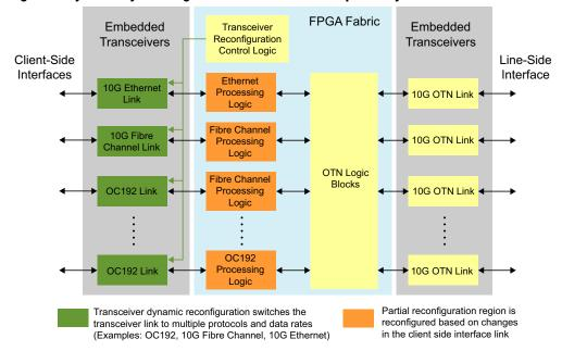
Figure 4. Dynamically Reconfigured Blocks in the OTN Muxponder System
