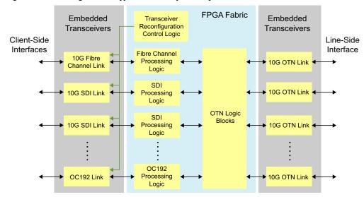
Figure 3. Block Diagram of a Typical OTN Muxponder System
