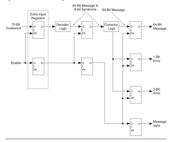
Figure 4. Decoder-Corrector Block Diagram
