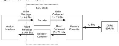
Figure 2. ECC Block Diagram
