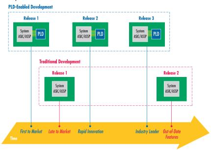
Figure 1. PLDs Complement Standard Devices
