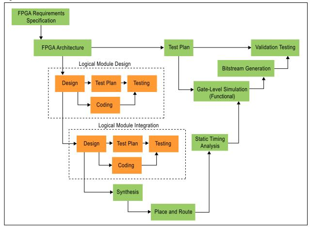
The V-Flow and the documentation that comes along with it maps all steps in the design of a safe application for FPGAs to the IEC specification and its requirements. In addition, it explains which tools should be used for the specified design steps. Specific chapters in the IEC specification guide the users to follow the right development steps for the development of a safe application.
