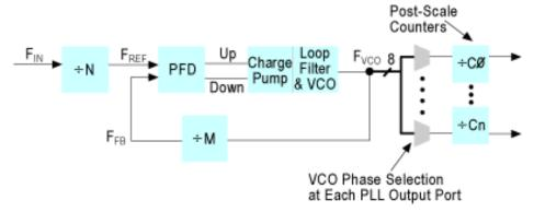
The analog nature of these PLLs provides very low jitter for a robust implementation of clocking schemes. Many configurable clock outputs allow tremendous flexibility for the system clock concept, as well as clock generation for the memory interfaces and I/O interfaces.
