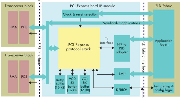
Figure 9. PCIe Hard IP Block
