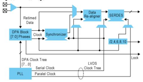
Altera's I/O pins support existing and emerging external memory standards such as DDR, DDR2, DDR3, QDRII, QDRII+, and RLDRAMII. They contain a self-calibrating data path, which constantly and dynamically adjusts itself to provide the highest reliable frequency of operation across process, voltage, and temperature. Other circuitry is included for alignment and synchronization, lane deskew, read/write leveling, and clock-domain crossing functionality.
