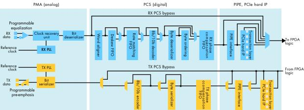
Figure 7. PMA and PCS Block Diagram
