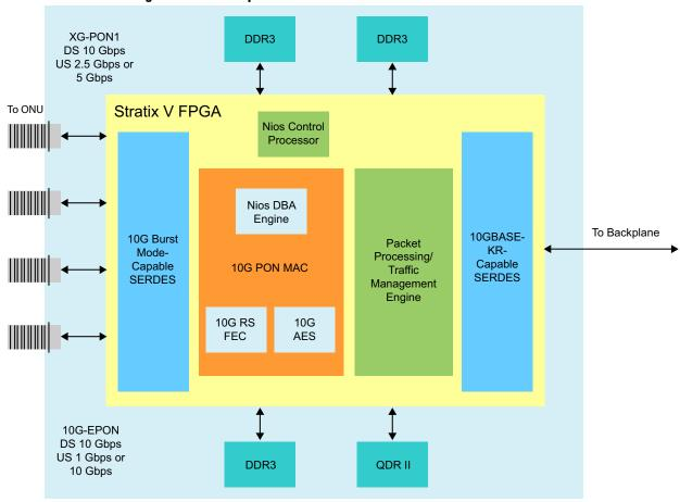
Figure 6. A One-Chip Solution for 10G PON OLT Enabled on a Stratix V FPGA
