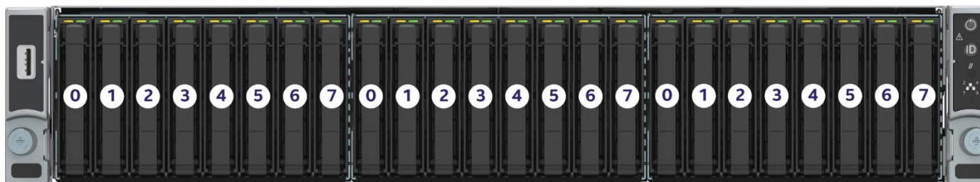
Figure 33. 2U 2.5" drive identification for each drive bay
