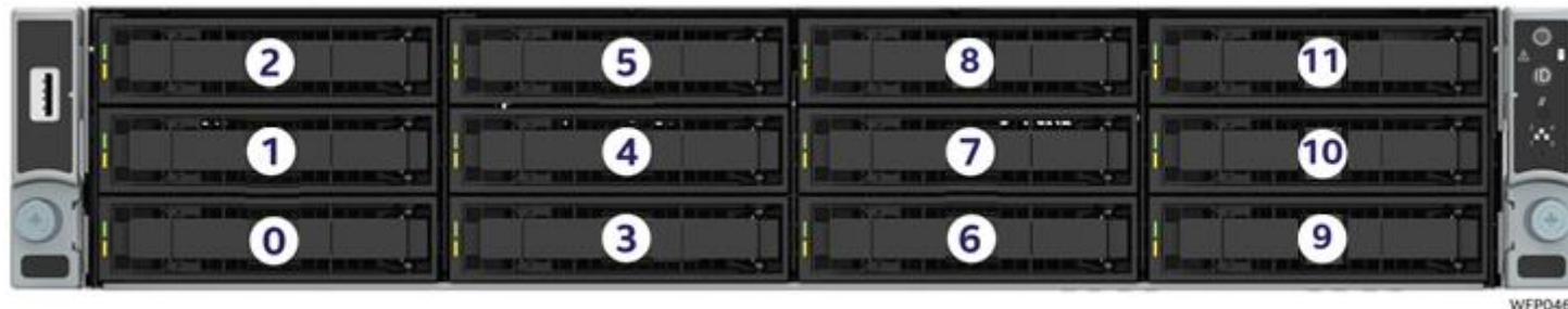
Figure 26. R2312WFxxx SAS/SATA backplane (NVMe support for drive 10 & 11 only)
