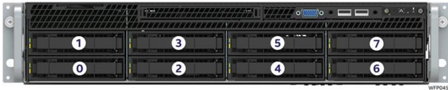
Figure 25. R2308WFxxx SAS/SATA backplane (no NVMe* support)
