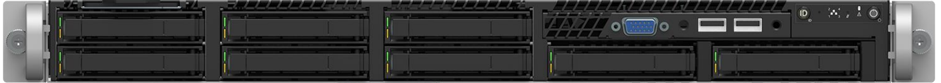
Figure 7. 1U, 2.5" x 8 drive configuration (Intel® Server System R1208WFxxx)
